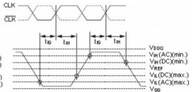
**Input Waveform Timing 2 ( $t_{IS}$ ,  $t_{IH}$ )**
