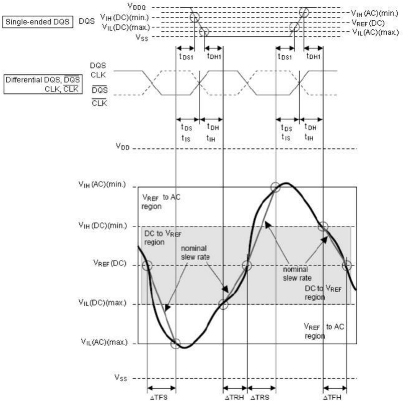
$$\text{Setup slew rate Falling signal} = \frac{V_{REF}(DC) - V_{IL}(AC)(max.)}{\Delta TFS}$$
