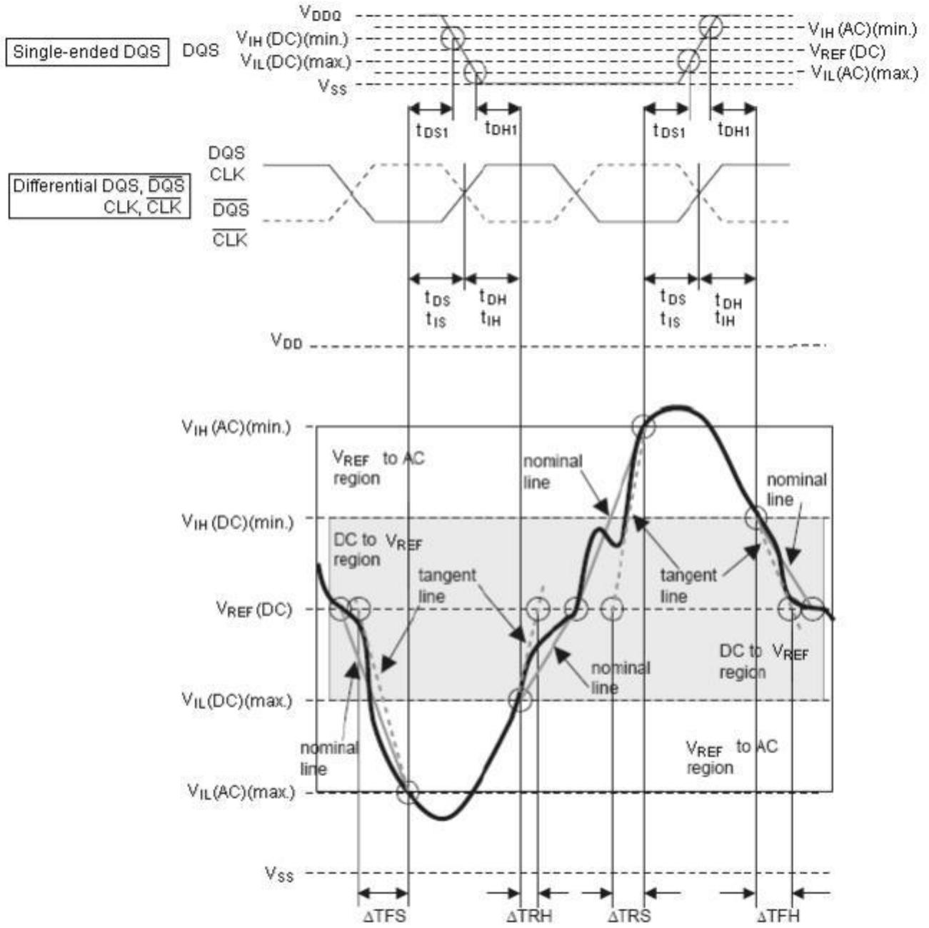
$$\text{Setup slew rate Falling signal} = \frac{\text{tangent line [ } V_{REF}(DC) - V_{IL}(AC)(max.) \text{ ]}}{\Delta TFS}$$
