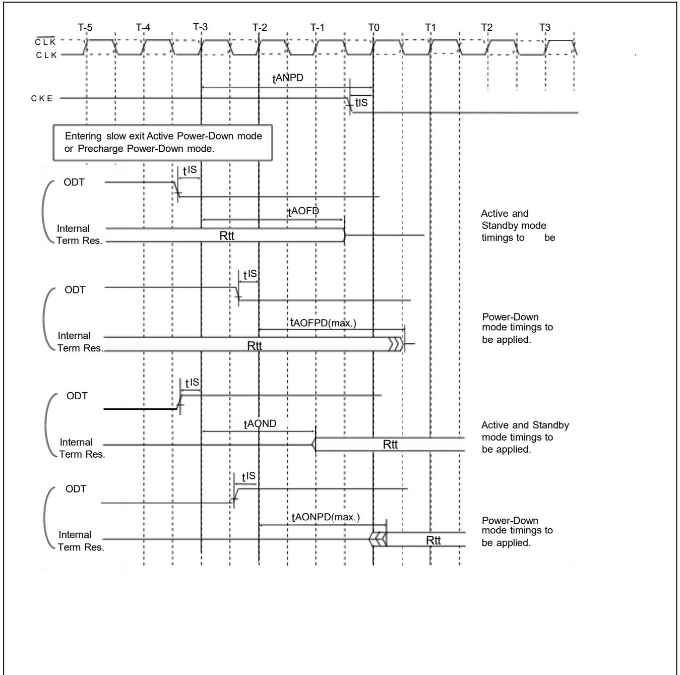
ODT Timing Mode Switch at Exiting Power-Down Mode
