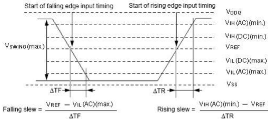
**AC Input Test Signal Wave forms**
