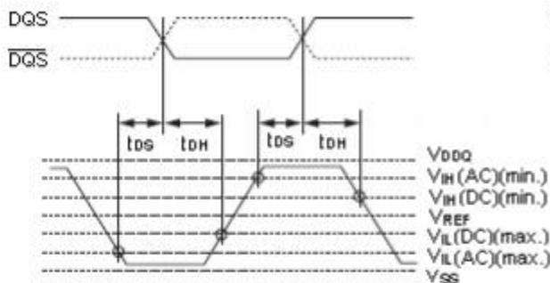
**Input Waveform Timing 1 ( $t_{DS}$ ,  $t_{DH}$ )**
